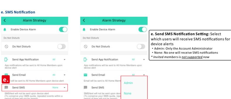
**e. Send SMS Notification Setting:** Select which users will receive SMS notifications for device alerts
